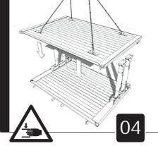
Using the four yellow handling points in the second panel, lift and lower the inverted panel onto the struts. Secure struts using Pin and 'R' clips.
