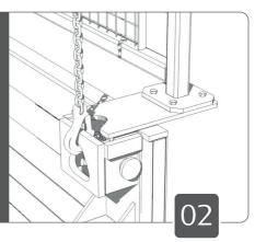
Attach a single heavy duty chain to each corner of the box in turn. Lift by no more than 150mm each time.
