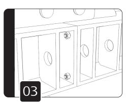
Complete the connection by securing two M24 lower bolts only. This prevents over-stressing of the blades during lifting and installation. These must be slackened off once installed.
