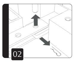
Re-connect the hoses between the Motorised Pump and the legs to depressurise the lower frame, then remove the corner pin and R-Clip.
