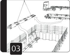
Using a certified 2 leg lifting chain, connect to the red lifting eyes. Lift and lower the first completed leg into place on level timber bearers.
