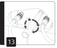
For each leg in turn, close the lockoff valve, return the pump lever to the neutral position and disconnect the hoses from the frame. Do not overtighten the lock off valve.
