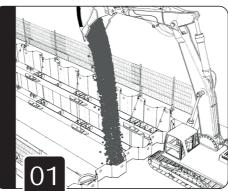
Backfill to the underside of the lower frame.
