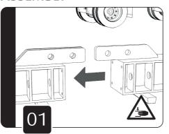
Assemble the extensions by sliding together the two blade connectors.
