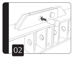
Align 2 two pin holes and connect the extensions by inserting the pin and R-Clips provided.
