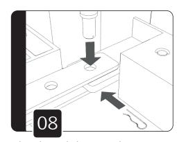
When the pin holes are in alignment, connect the two legs using the corner pin and R-Clip provided. Repeat this process to connect the remaining corners.
