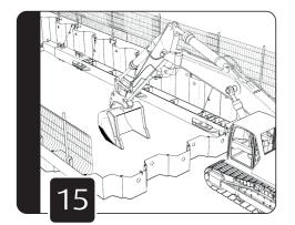
Continue excavation to the second level position as stated on the scheme specific design. If 'dig and push', progressively drive sheets as the excavation continues.
