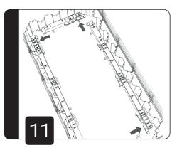
Expand and connect the remaining legs using the corner pins and R-Clips.
