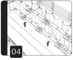
Once the legs are disconnected, they can be lifted clear of the excavation. Take care to avoid striking the upper frames when lifting through.
