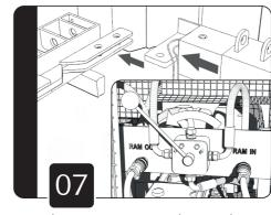
Start the pump engine and move the lever to the 'ram out' position to expand the hydraulic leg. Note: If the leg retracts, swap the hoses over on the pump and continue.
