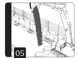
Continue backfilling and compacting to the underside of the top frame.
