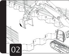
Connect edge protection as required and excavate to a depth of approximately one metre or 200mm below the required
