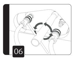
Attach the opposite end of the hoses to the two couplings on the hydraulic leg. Use the tool provided to open the lock off valve by turning it anti-clockwise.
