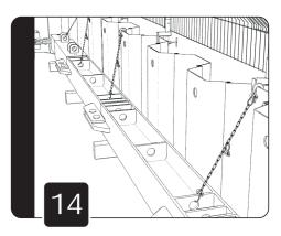
Attach the restraining chains provided between the hanging points on the frame and the top of the sheets at the locations specified in the scheme specific drawings.
