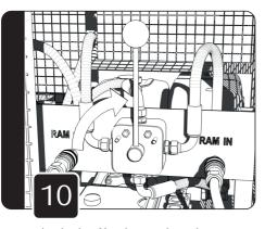
Once the lock off valve is closed, return the lever on the pump to the central neutral position.
