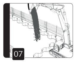
Reinstatement can then continue to ground level. Remove any edge protection and ladder access and withdraw the trench sheets using appropriate equipment.
