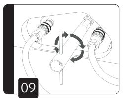
Close the lock off valve by using the tool provided to turn clockwise. Do not overtighten.
