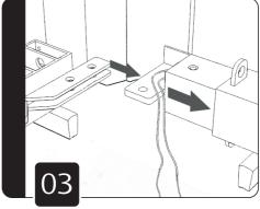
Continue depressurising to fully separate the legs, setting the pump to the 'ram in' position. Repeat this process for the remaining corners.
