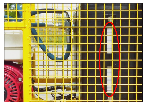
Shoring Fluid level indicator (circled red)
