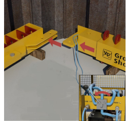
8. Start the pump engine and move the lever to the 'ram out' position to expand the hydraulic leg. Note: If the leg retracts, swap the hoses over on the pump and continue.
