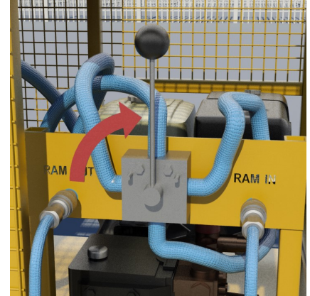
11. Once the lock off valve is closed, return the lever on the pump to the central neutral position.
