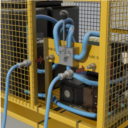
6. Attach both hydraulic hoses to the 'ram out' and 'ram in' coupling on the Motorised Pump.
