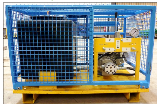
The Hydraulic Oil Motorised Pump is housed in a BLUE CAGE
