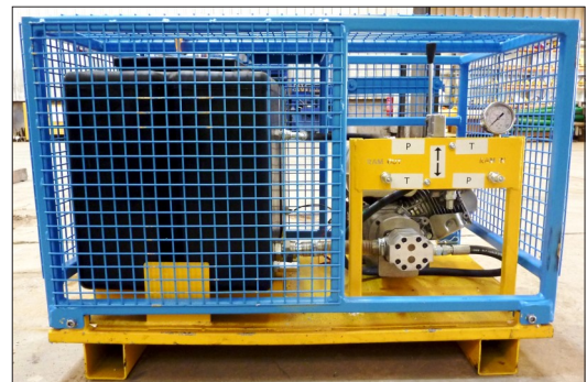
The Hydraulic Oil Motorised Pump is housed in a BLUE CAGE
