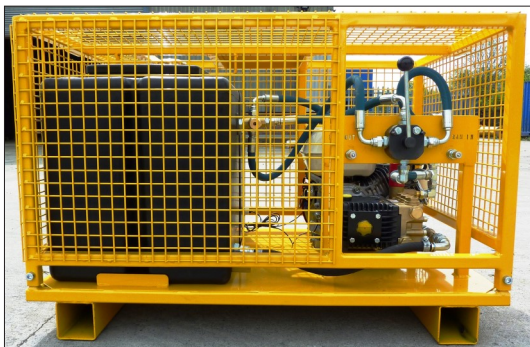
The Shoring Fluid Motorised Pump is housed in a YELLOW CAGE
