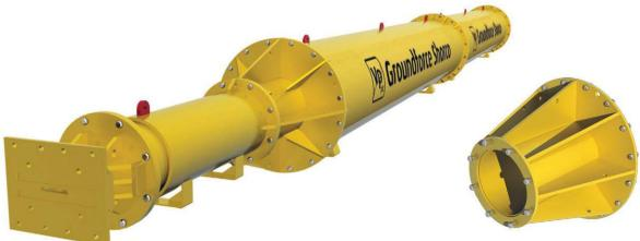
To connect the standard extensions and the hydraulic ram (all 610mm dia) to the larger "Super" Extensions (1220mm), a 1.0m long tapered adapter piece is utilised. For each strut assembly, two adapter pieces are required.
