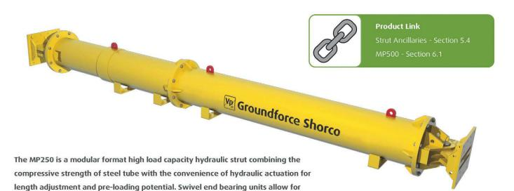
MP250 struts use 610mm diameter tubular sections as the main structural member. At shorter spans, the hydraulic capacity limits the axial load and at longer spans, the potential for flexural buckling of the extension sections dictates overall axial capacity.
